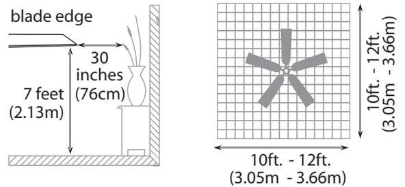
This fan can be mounted as a **flushmount** on a regular (no-slope) ceiling *only*. **Downrod** installations are **not** available for this fan.
